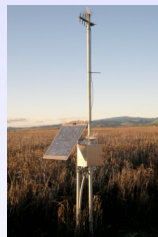
Figure 1. Telemetry station providing real-time data from CTDS channel moorings
